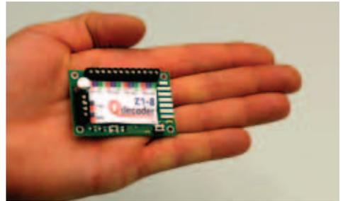
***Qdecoder** are fully compatible with all DCC and Märklin-Motorola systems. **Qdecoder** can be used in analogue model railways too due to their sequence control capacities.*
